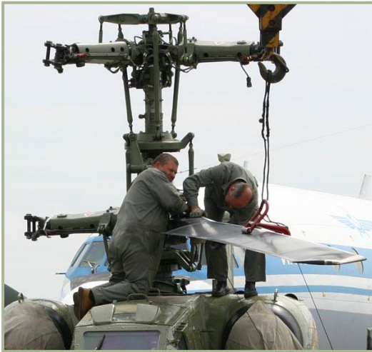
1-4: Assembly of main rotor
