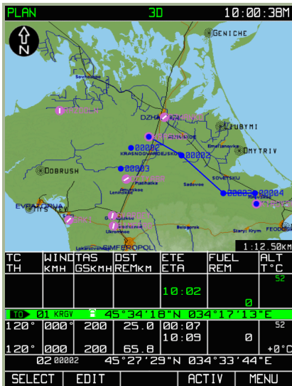
3-71: Loaded route before inverting
