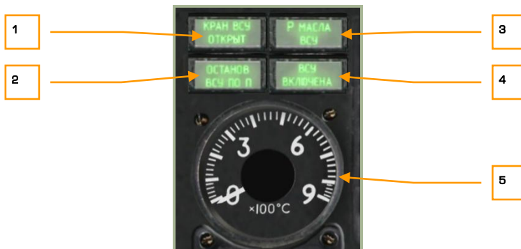
2-78: Auxiliary Power Unit (APU) panel
