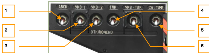
2-53: Radio and data link power control panel
