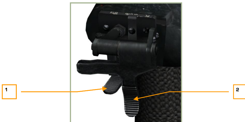
2-6: Weapon (large) and Cannon (small) triggers in default position – Release Weapon trigger operates
