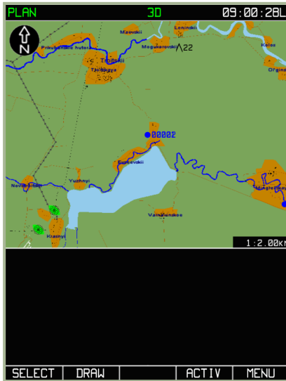
3-28: View of the PLAN sub-mode after unloading of current plan
