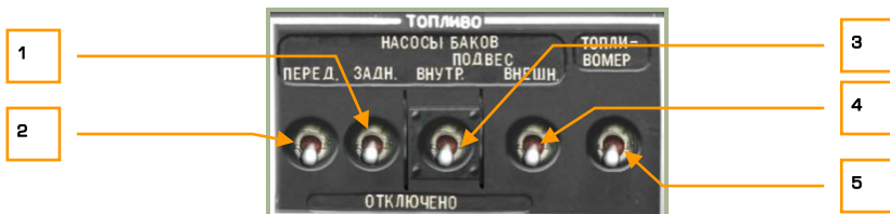
2-54: Fuel pump controls
