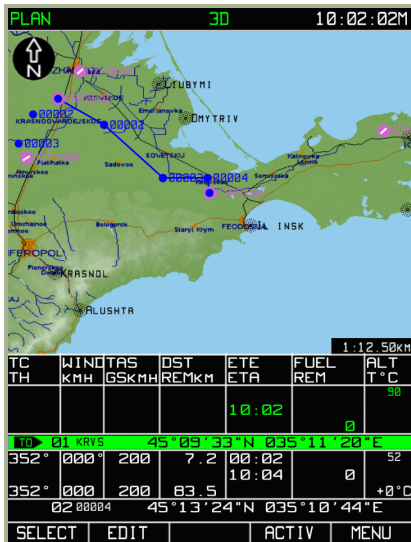
3-73: Result of inverting route
